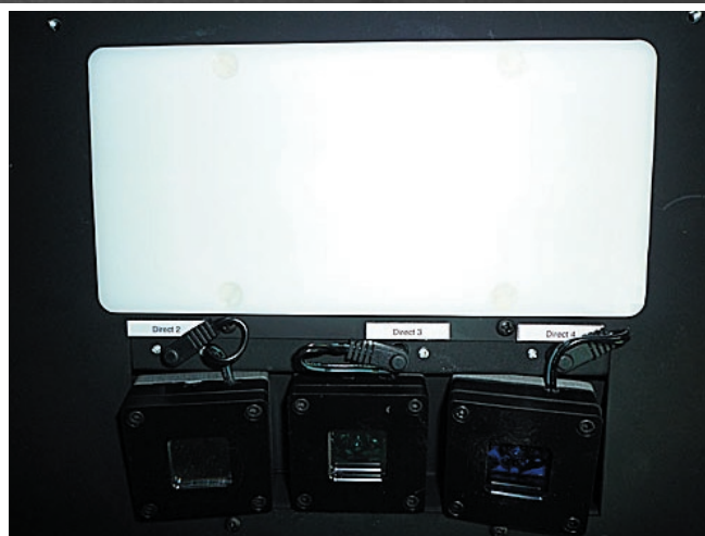
Figure 5b Interior left side of Luminary/FX darkroom with full LED module bank
