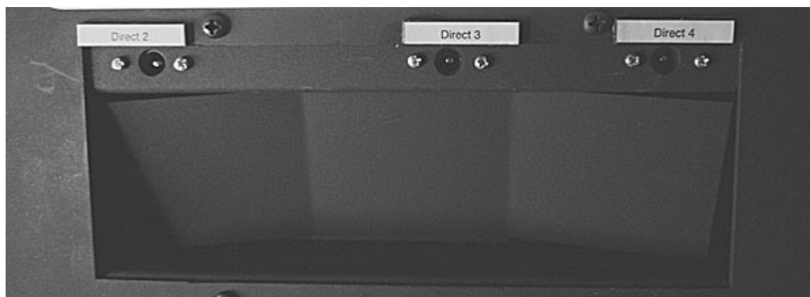
Figure 5b Interior left side of Luminary/FX darkroom with full LED module bank
